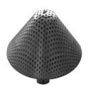
A **perforated filter** inverted cone shape (graspo) and **removable**, placed on the funnel bottom, **retains impurities and other dirt**, allowing more water to pass through it. The **nozzle**, placed under the funnel, is **dimensioned** in such a way as to ensure a constant water flux regulation **in case of sudden rainfall of high intensity**, decreasing the reason of a typical error of the rain gauges in this condition.
