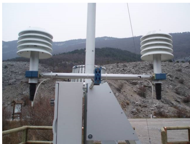
Picture 14 – Particular of the terminal support fixed to the main support
